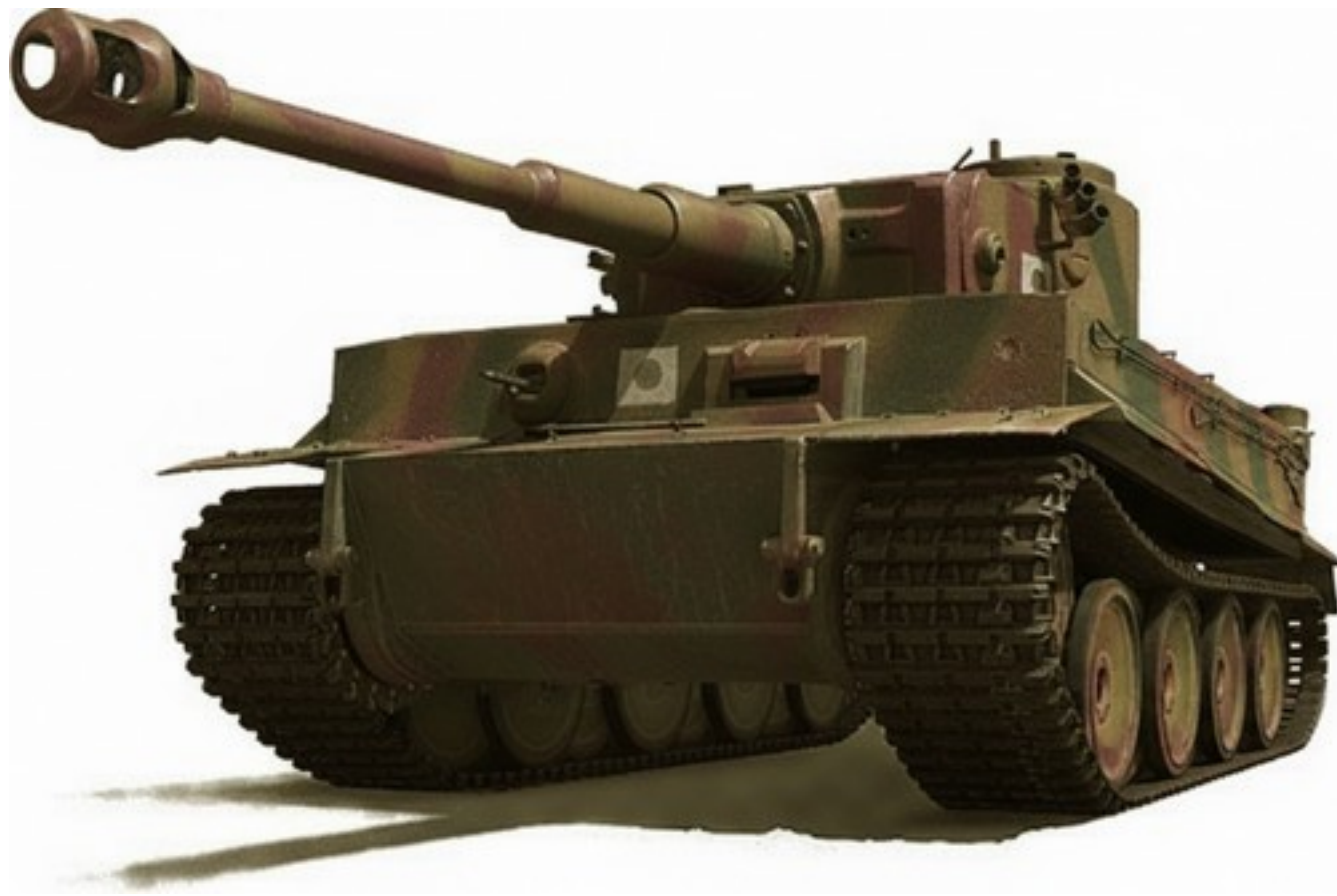
TIGER 1: 0.48 mpg on-road*, range 80 mi. 57 tonnes, 1,354 specimens produced.
