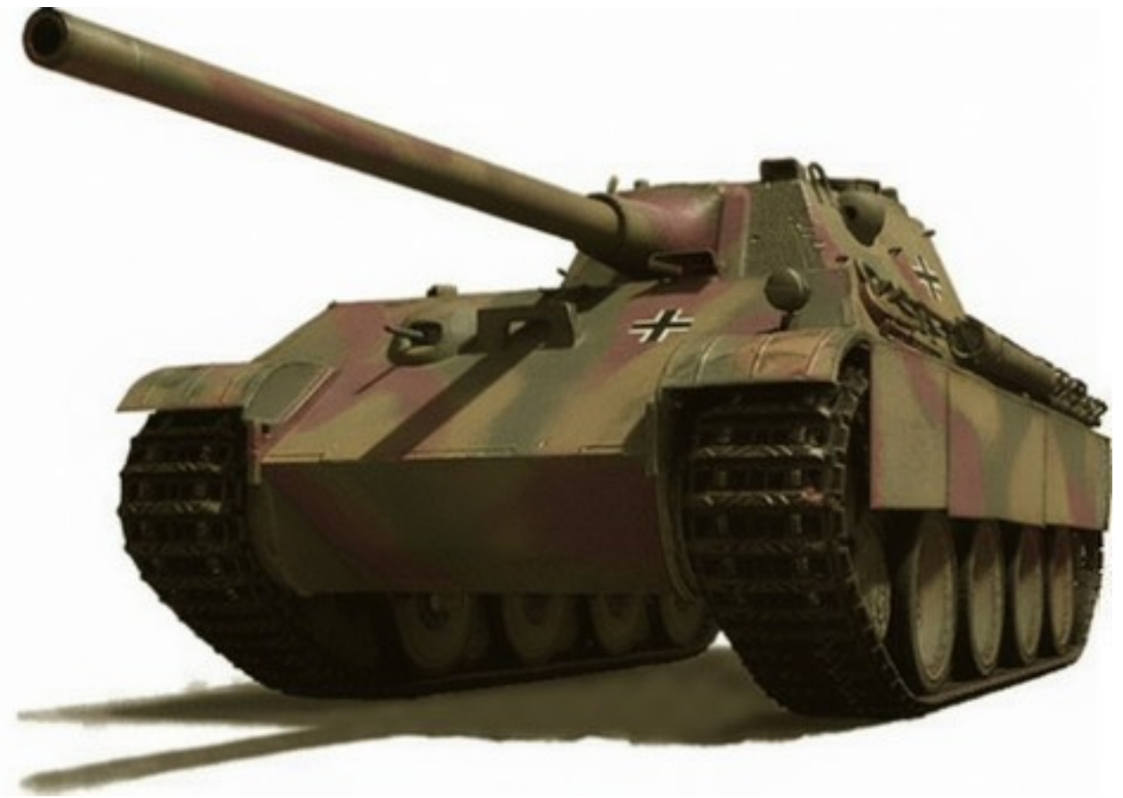
PANTHER: 0.84 mpg on-road*, range 150 mi. 46 tonnes, 5,508 specimens produced.
